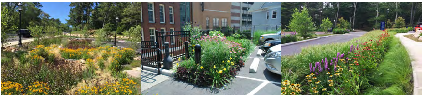
These landscaped areas treat stormwater and can be integrated into designs for safer walking, biking and parking.
